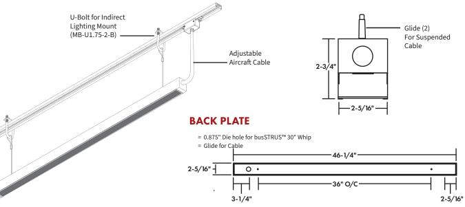
\*Indirect linear fixtures connect to the busSTRUT via the provided Aircraft Cable, which is then attached to the U-Bolt (MB-U1.75-2-B).
